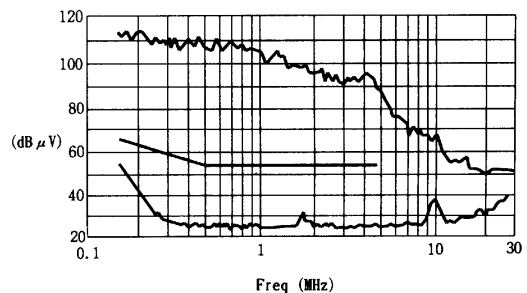
European Standards EN55011 Class B measurement data
